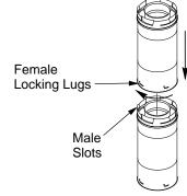
Figure 8 - Vent Pipe Connections
